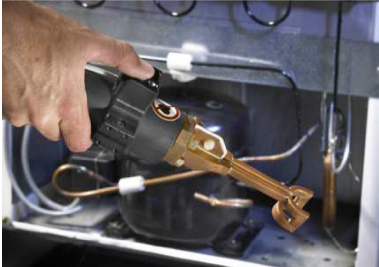
The right heat just where it's needed. A hand-held transformer fitted with a customized coil makes it easy for the operator to deliver the benefits of fast, clean, accurate induction brazing.
