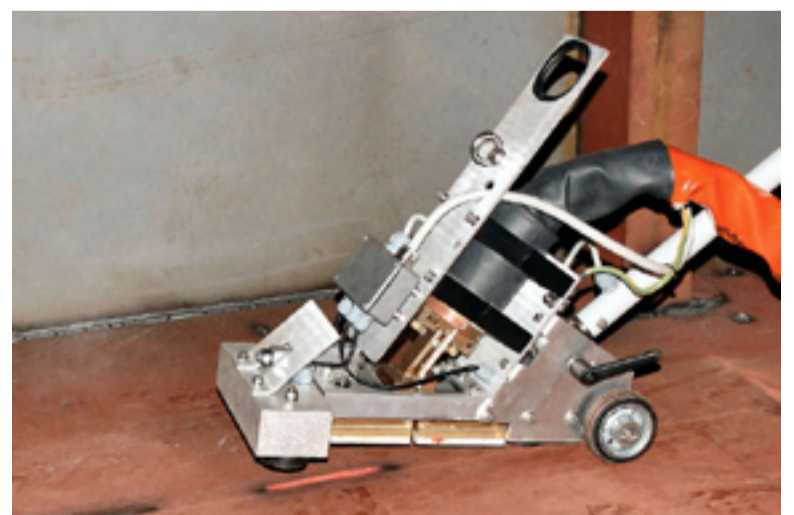
Induction heating is controllable. The result is faster, better quality fairing than that achieved by open flames.
