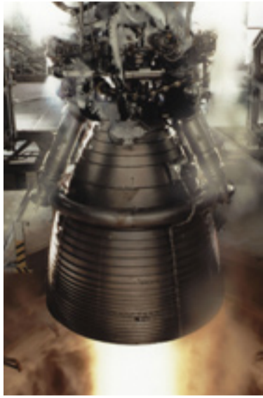
Vulcain engines are used on the European Space Agency's Ariane 5 rockets. The lightweight engine cone is made from graphite produced using induction heating.
