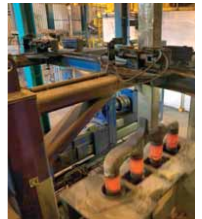
No dust, no fumes, no noise. An EFD Induction heater gets to grips with a 170 mm anode stub.
