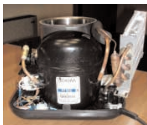
Good enough to eat. Induction heating brazed the joints in this ice-cream maker compressor.
