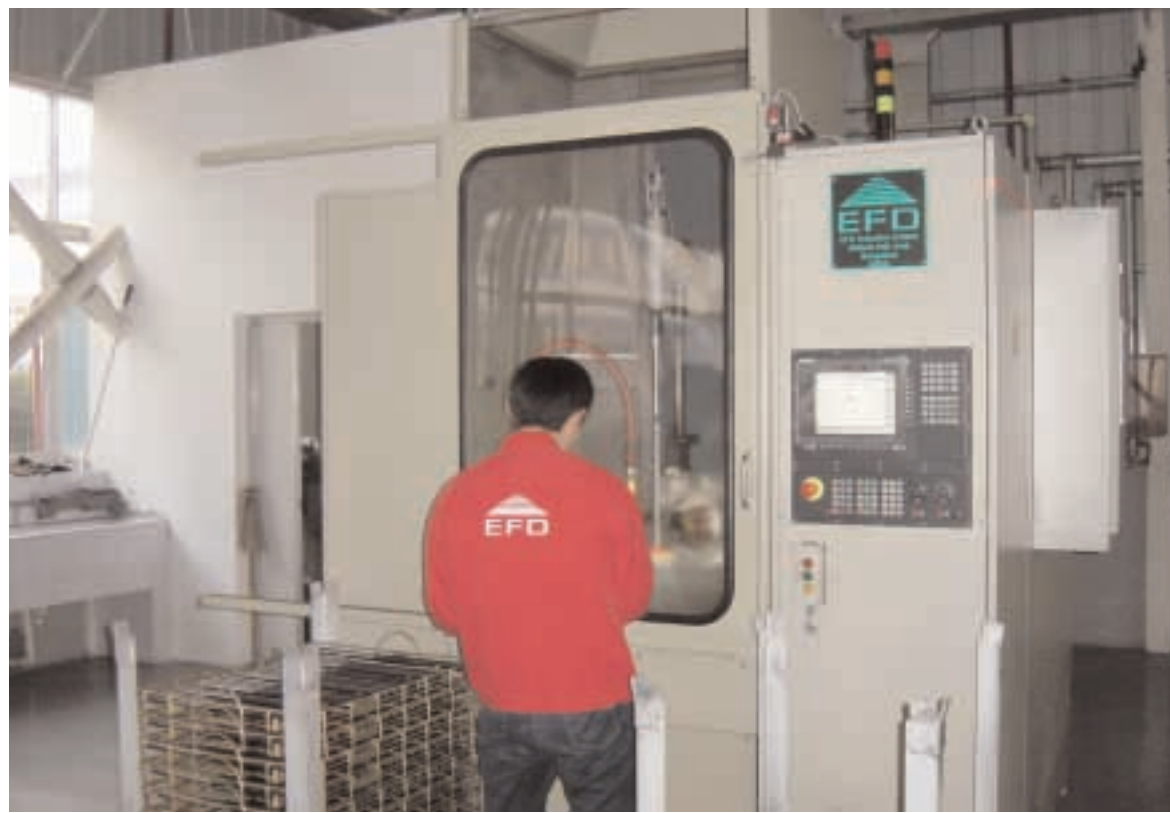
Fine-tuned for success. An engineer at EFD Induction (Shanghai) works on an induction hardening machine.
