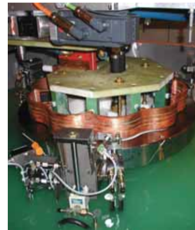
The working station of Hägglunds Drives new hardening system from EFD Induction. Note the possibility to quench the cam rings by quench shower or agitated bath.
