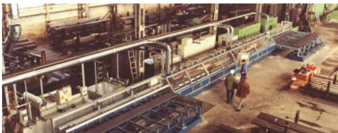
A typical installation for induction heat-treatment of steel bars.
