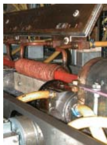
Temperature supervision by pyrometer ensures controlled heating.
