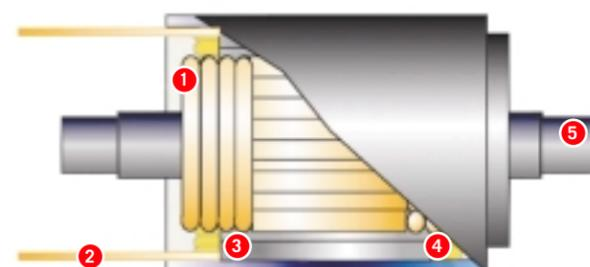
1. Rotor 2. Connection wires 3. Magnet 4. Stator 5. Axle shaft
