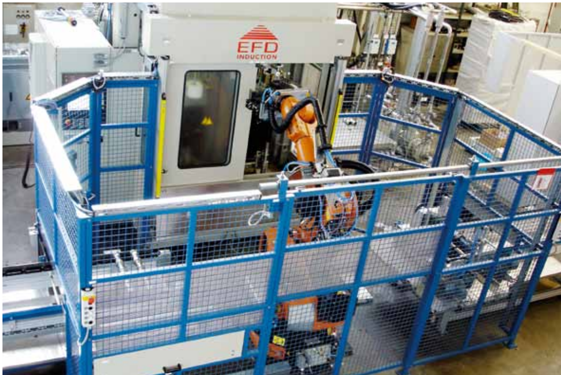
Many HardLine vertical machines are customized to work with robotic handling solutions. Above, a HardLine machine and its robotic handling system near completion at the EFD Induction factory in Freiburg, Germany.
