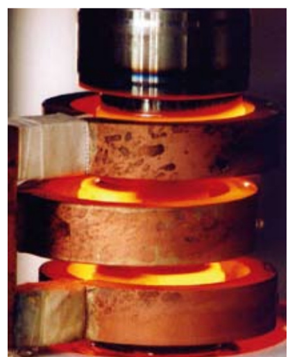
EFD Induction package hardening in action. Each coil operates independently and is formed to match a specific coil.
