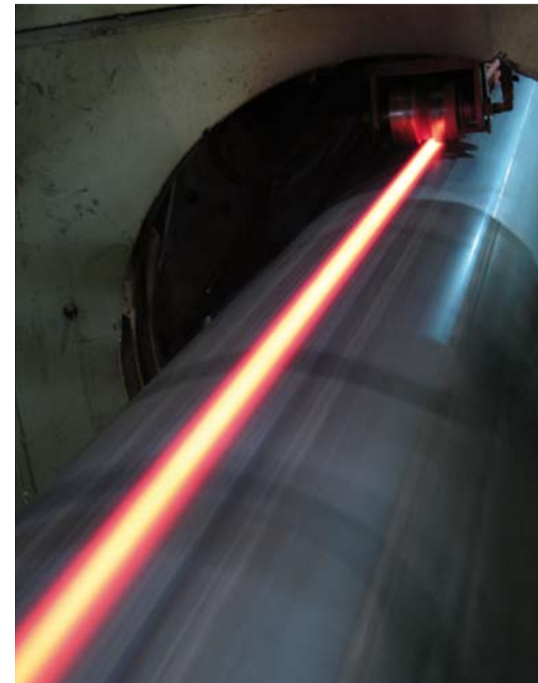
A 2,400 kW EFD Induction seam annealer in action. The orbital tracking system is fully automated.
