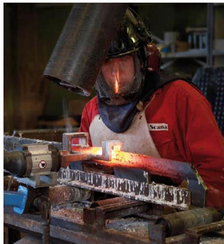
Norway's Scana Steel replaced rotating converters with an EFD Induction Sinac 25/40 Twin. Output increased dramatically.
