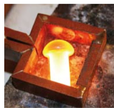
A rivet is heated to 1100°C in 7 seconds, consuming only 0.03 kWh.
