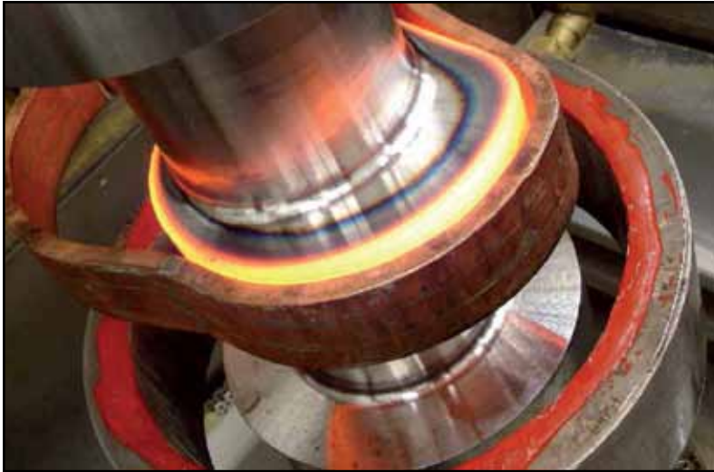
Left: EFD Induction single cam hardening with special coil BELOW: EFD Induction package hardening
