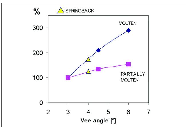
Figure 5: Melting vs. Vee angle; 200 kHz, 14.6m/min
