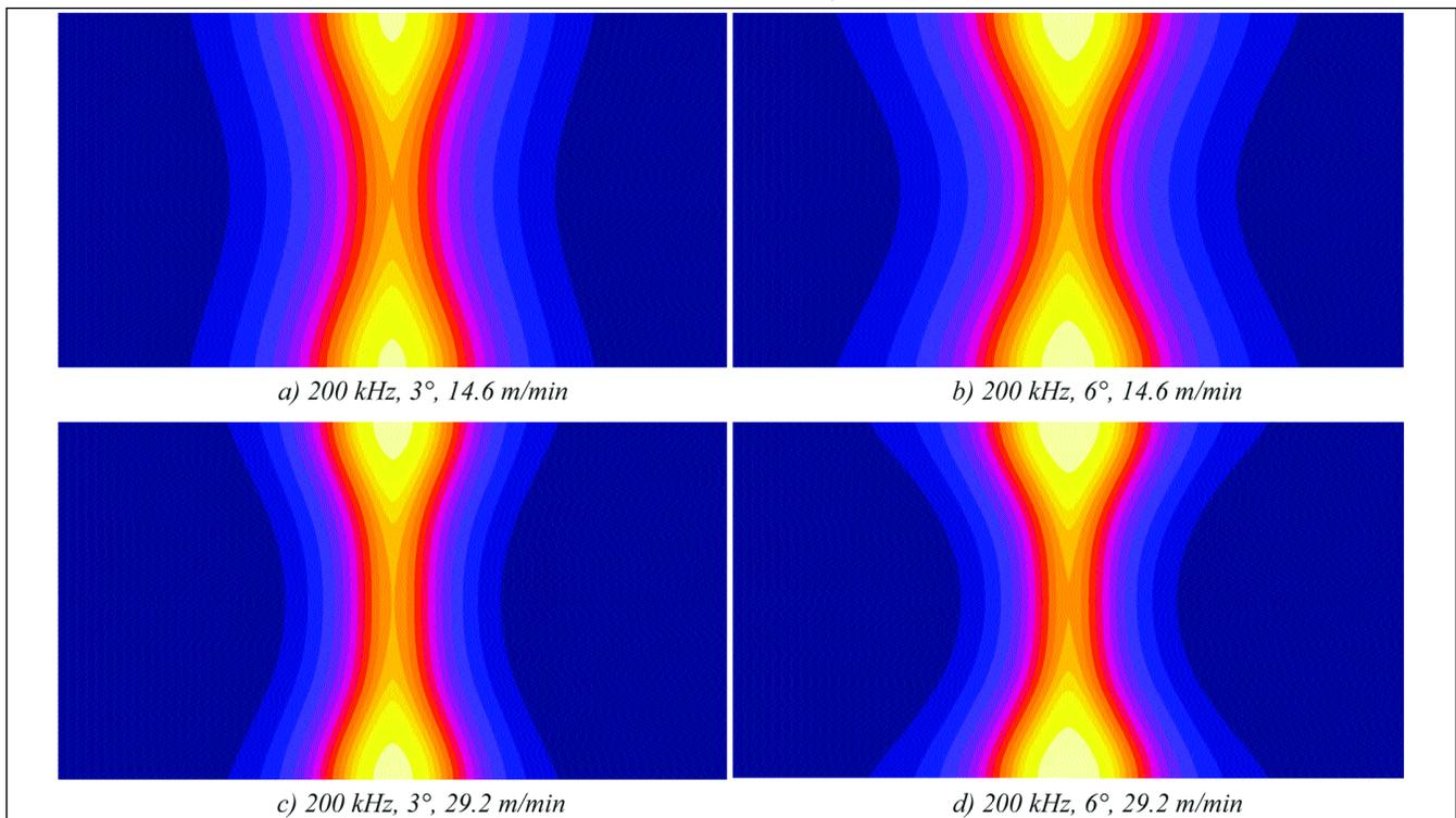
Figure 2: Temperature distribution at the weld point
