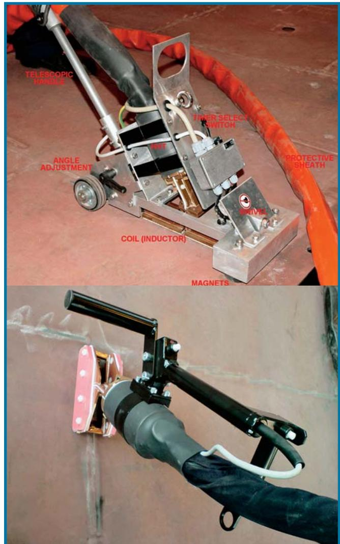
Fig. 2. Terac induction heating options: (a) Terac heating unit for straightening decks and (b) Terac heating unit for straightening vertical bulkheads.
