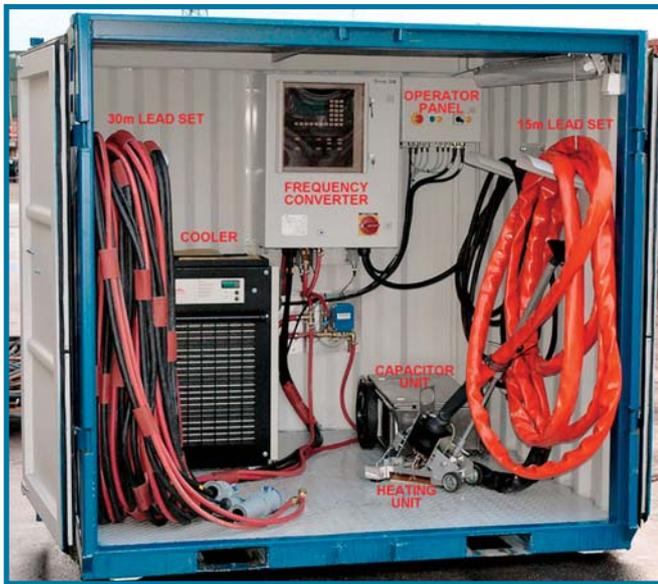
Fig. 1. Main components of the Terac heating system.
