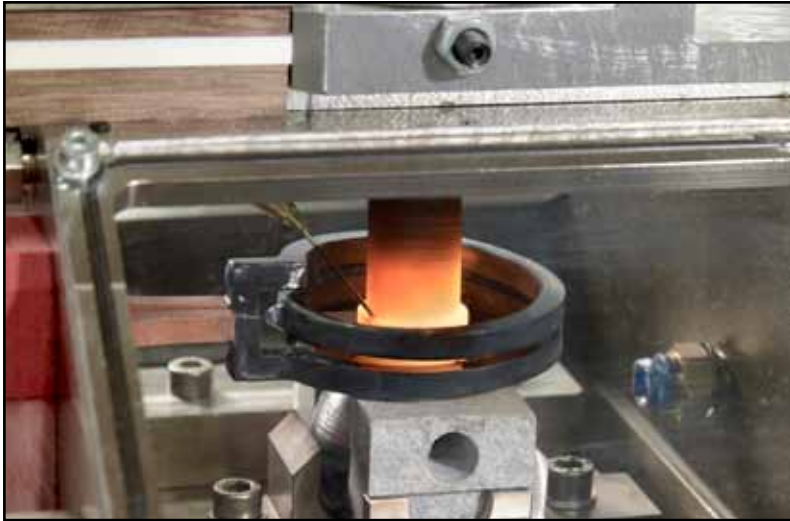
LEFT: A close-up of the brazing solution in action. The induction coil, which is dual-turn with an inner diameter of 42mm, handles various dimensions of banjo fittings ranging from 5-18mm in diameter. BELOW: The end result. Exceptionally clean banjo fittings brazed in a flux-free protective atmosphere.
