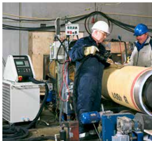
An EFD Induction mobile Minac system in action in the offshore industry. In this photo the power being applied to the workpiece is controlled by an easy-to-use handheld transformer.
