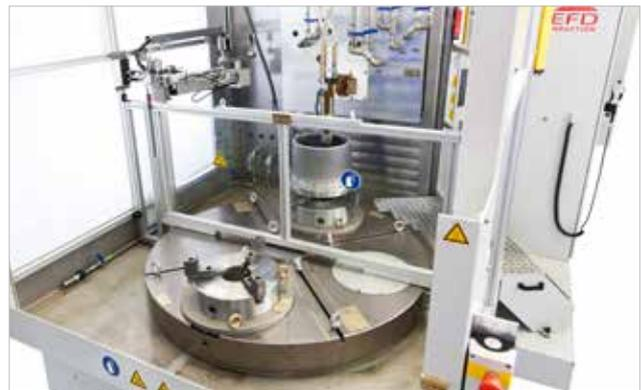
*Flexibility to suit your needs—this indexing table on a HardLine VL 1000 system can be manually or automatically loaded.*
